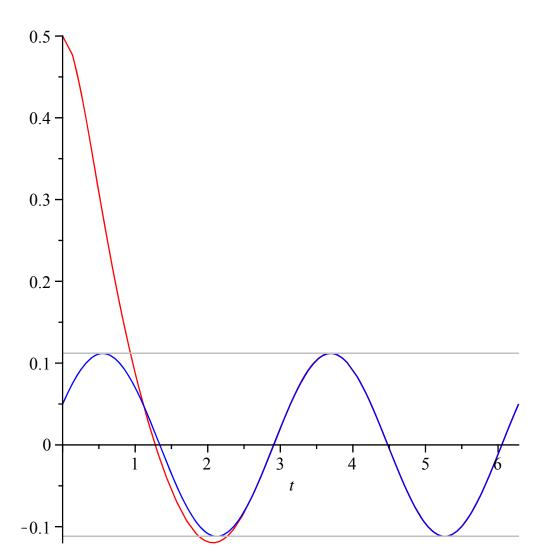
The calculated amplitude (gray horizontal lines) indeed describes the steady state solution (blue).
